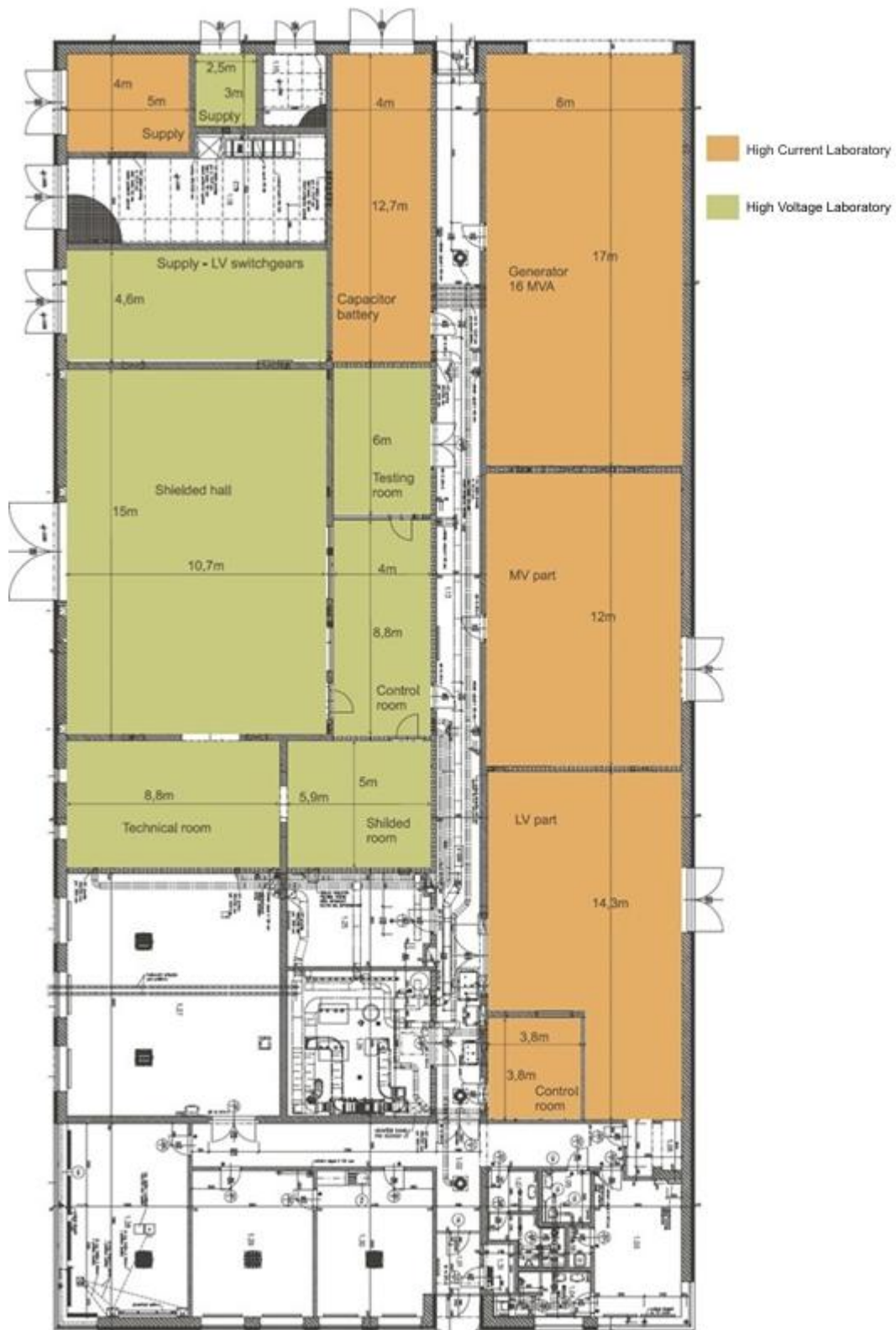
Fig. 7 Ground plan of CVVOZEPowerLab building
